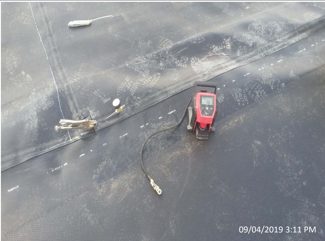
Photo 54- Geomembrane Non-Destructive Seam Air Pressure Testing
